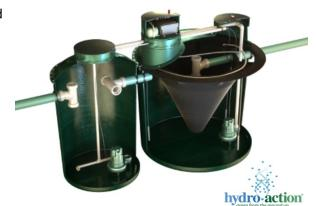
denitrification. Treated wastewater exits by gravity through a tee structure located in the center of the clarifier, and treated effluent is then discharged to the leaching structure.
